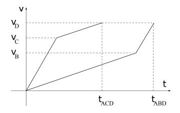
Path 2 (ACD): the free fall occurs first, so the sphere gets rapidly accelerated and reaches C at a high velocity. The acceleration from C to D is small but due to the high velocity the distance is covered fast.
