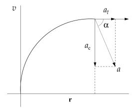
figure. So it is necessary to determine the tangential acceleration. Since the acceleration has the biggest value at the exit of the curve only this point needs to be investigated. The covered distance  $s_1$  is:
