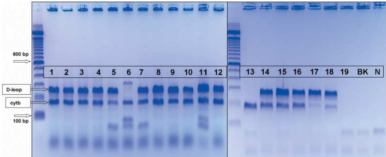
Fig. 1 Negative image of a SYBR-Green stained, 2% agarose gel of co-amplified PCR products. Samples 1–19 represent DNA samples extracted from ancient salmon remains, BK is the blank extract and N is the PCR negative control. Sample 19 displays amplification failure of both bands, while sample 13 displays amplification failure of the longer D-loop fragment. The markers on the left are 100-bp ladders (from Invitrogen).
