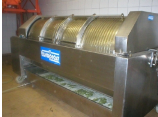
Fig. 8: A modern hydraulic winepress.
