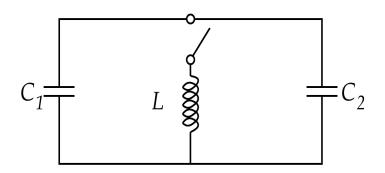
A resonant circuit consists of an ideal coil L = 2,5 mH and the capacitors  $C_1 = 2 \mu \text{F}$  and  $C_2 = 3 \mu \text{F}$ . The capacitors were charged with U = 180 V. Then, the switch is closed.
