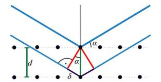
The maxima in the measured spectrum occur when the maxima of the reflected light waves (at different planes) are superimposed. This happens e.g. at  $\alpha \approx 7.5^{\circ}$ . So here the path difference  $2\delta$  must correspond exactly to the wavelength  $\lambda$ :
