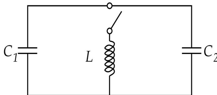
A resonant circuit consists of an ideal coil  $L = 2,5 \text{ mH}$  and the capacitors  $C_1 = 2 \mu\text{F}$  and  $C_2 = 3 \mu\text{F}$ . The capacitors were charged with  $U = 180 \text{ V}$ . Then, the switch is closed.
