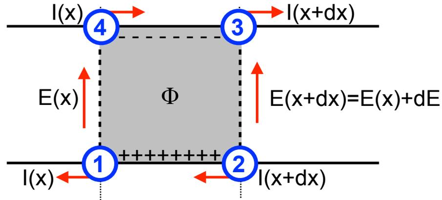
$$\frac{\partial}{\partial t} (2) \rightarrow \frac{\partial^2 u}{\partial t \partial x} = -L^* \frac{\partial^2 I}{\partial t^2} - R^* \frac{\partial I}{\partial t}$$
