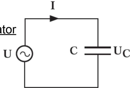
$$\begin{aligned}U &= U_0 \cos \omega t \\ \text{Kirchhoff: } U - U_C &= 0 \\ \dot{U} &= \frac{1}{C} \dot{Q} = \frac{1}{C} I \\ -\omega U_0 \sin \omega t &= \frac{1}{C} I \\ I &= -\omega C U_0 \sin \omega t\end{aligned}$$
