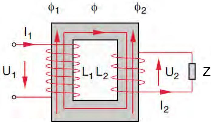
$$\underline{Z}_{\text{trafo}} = \underline{U}_1 / \underline{I}_1 = \text{????}$$
