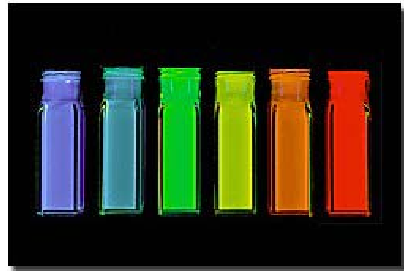
A family of Qdot particles can be made to emit a full spectrum of colors when excited with a single excitation source.
