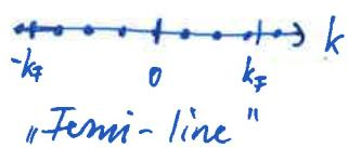
number of transverse modes:  $\underline{\underline{M}} \approx \frac{2k_F}{\Delta k} = \frac{2k_F L_x}{T} = \frac{k_F L_x}{\pi}$
