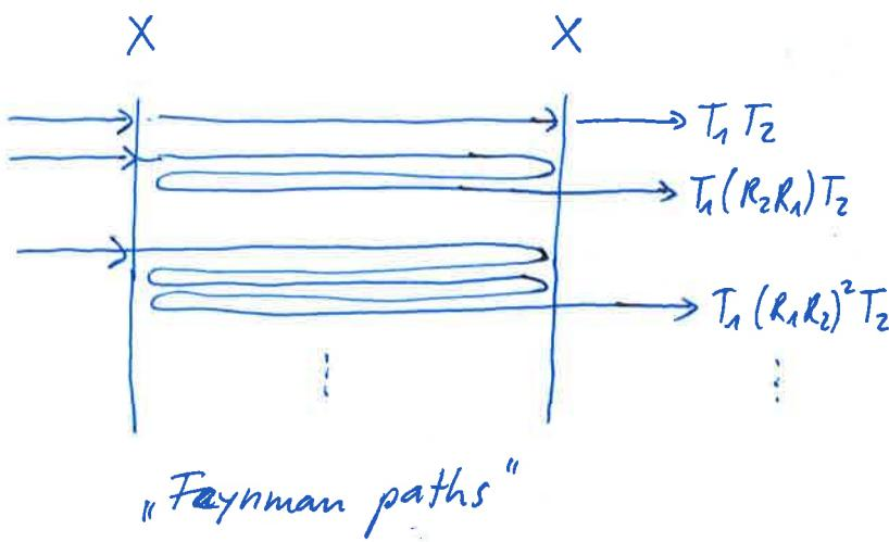
$$\begin{aligned} \underline{\underline{T_{12}}} &= T_1 T_2 \cdot \sum_{n=0}^{\infty} (R_1 R_2)^n \\ &= \frac{T_1 T_2}{1 - R_1 R_2} \\ &\uparrow \text{geometric series} \\ &= \frac{T_1 T_2}{1 - (1-T_1)(1-T_2)} \end{aligned}$$
