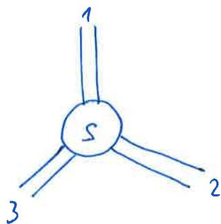
Determine the scattering matrix  $S$  ( $3 \times 3$ ).
