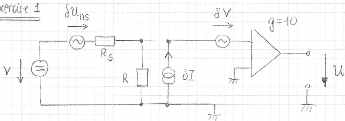
$$\left. \begin{array}{l} \delta U_{ns} = \sqrt{S_{ns}} \\ \delta I = \sqrt{S_I} \\ \delta V = \sqrt{S_V} \end{array} \right\} \text{where } S_V, S_I \text{ and } S_{ns} \text{ are special noise powers} \\ (\text{amplifier has infinite input impedance})$$
