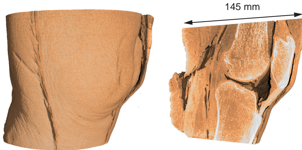
Figure 8. 3D rendering of a tomogram of an entire human knee with a specimen diameter of 145 mm. Despite the specimen size, the trabecular structure of the bone can be resolved.
