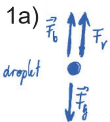
Forces: gravitation:  $|\vec{F}_g| = mg = \rho_{oil} \cdot V_{drop} \cdot g = \rho_{oil} \cdot g \cdot \frac{4}{3} r^3 \pi$
