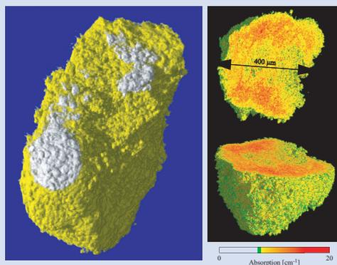
The cluster of  $10^4$  to  $10^5$  HEK 293 cells about 0.5 mm long shows that SR $\mu$ CT might uncover cell-like structures. The white areas instead of the yellow color should support the impression. The data are visualized from a tomogram obtained at the materials science beamline 4S (SLS, PSI, Switzerland) using the photon energy of 10.0 keV. To increase the density resolution (contrast) the data are binned by the factor of 3.
