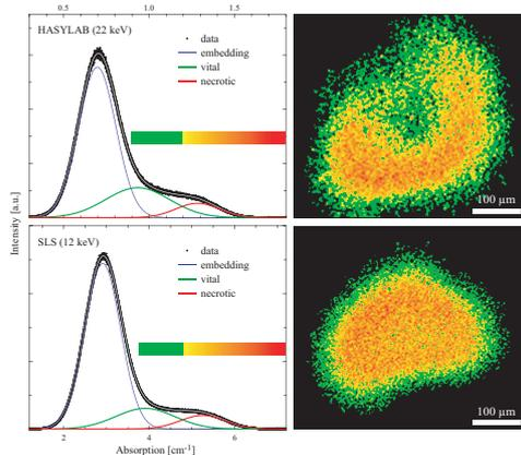
The RNA/DNA staining using osmiumamine-B results in a transition range, green colored, which is related to the area at the cluster's periphery about 50 to 100  $\mu$ m wide.
