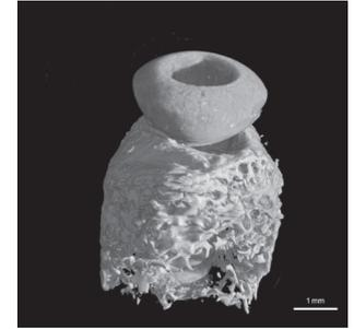
The corrosion behaviour of cortical bone screws was analyzed using SR $\mu$ CT at a photon energy of 30 keV. The screws, machined from magnesium alloy AZ31 extruded rods, were implanted into hip-bones of sheep and removed three months later.
