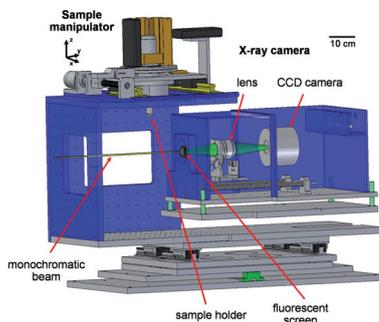
Schematic of the microtomography apparatus in absorption contrast mode. The incident monochromatic X-ray beam penetrates the sample and hits the fluorescent screen, where it is converted into visible light, which then is projected onto the CCD camera.
