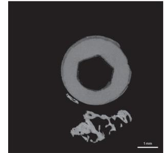
While the screw head exhibited severe surface corrosion on the convex areas of the screw head (see 3D figure and axial cut above), just minor corrosion attack was observed on the area of the machined hexagonal screw drive. The threads of the screw displayed a quite homogeneous corrosion layer (see frontal cut below) [4].
