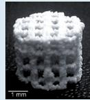
An optical image of the surface of a 3D-printed and collagen-coated scaffold intended for use as bone replacement. These scaffolds are individually designed according to the information determined by a CT scan of the bone.
