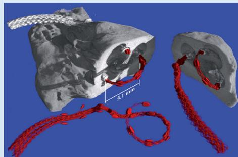
The cochlear implant consists of 12 electrodes and was inserted into the inner ear of a patient with a sensory neural hearing loss. The non-destructive visualization of the integration of the implant inside the inner ear using SR $\mu$ CT is almost free of any artefacts, which are often unavoidable using histological techniques [3].
