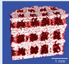
The virtual cut of the scaffold is colored according to the fitted histogram: air – black, coating – red, and HA – white. The collagen coating is homogeneously distributed on the surface filling the open micro-pores of the HA, while the macro-pores remain open.
