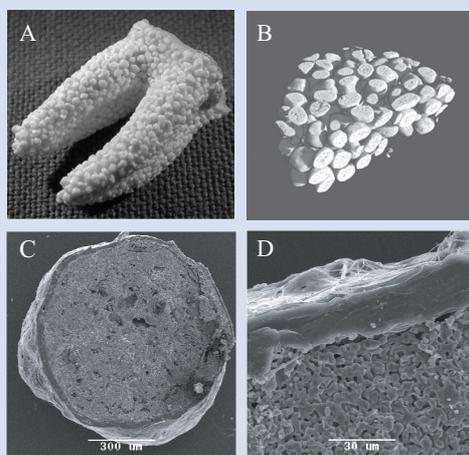
RootReplica<sup>TM</sup> is an exact copy of a tooth root (A) that provides an open porous structure (B,  $\mu\text{CT}$  image) where the individual granules (C, SEM picture) are fused together by the polymer layer that covers each granule (D, SEM picture). The scaffold shows an interconnected macroporosity among the granules, as well as a microporosity within each granule.
