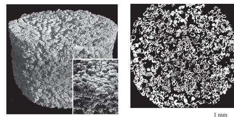
$\mu\text{CT}$  and SEM image (inset) of the outer shape of a PLGA scaffold on almost identical scale (left). The images demonstrate the complex structure of the porous sample. Slice of the tomograph obtained from the PLGA scaffold (right). The image was obtained after thresholding and filtering the binary data.
