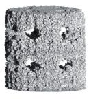
3D reconstruction of  $SR\mu CT$  dataset of a 3D printed HA-scaffold
