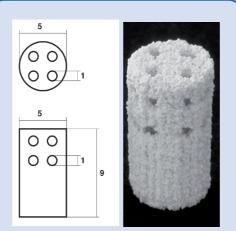
Design of the 3D printed scaffolds used in this study. The right image shows the 3D printed scaffold after sintering.
