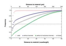
Porosity (distance to material) of 3D printed HA-scaffolds. The open triangles represent the trend of the whole scaffold where the other curves show information of the three ROIs.
