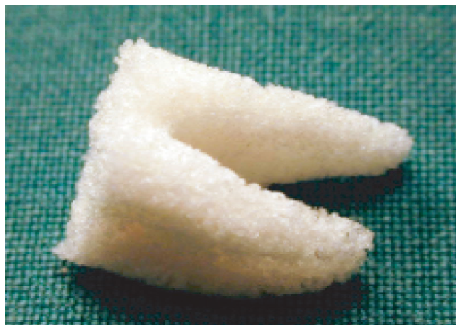
Figure 2. Root replica obtained by consolidation of PLGA fibers under carbon dioxide pressure at room temperature. The length of the root is about 15 mm. [Color figure can be viewed in the online issue, which is available at www.interscience.wiley.com .]
