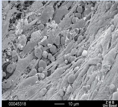
Scanning electron microscopy image of a pore of the generated construct following in vitro culture. The ceramic pore is filled with a stromal-like tissue, consisting of a 3D-network of heterogeneously shaped cells and extracellular matrix.
