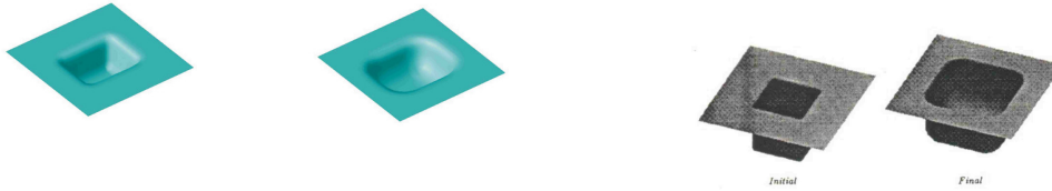
Figure 3.29: Surface evolution during isotropic etching (left) in comparison with Adalsteinsson and Sethian [4] (right)
