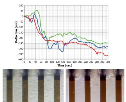
efore after otime Trypsin/EDTA was injected at times 40 s untill times 260 s and a fast release of cellular forces on three different cantilevers was observed. Before and after the experiment the cantilever array was observed under the microscope to
