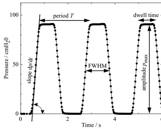
Fig. 2. A sequence of cough or Valsalva profiles are characterised by the period  $T$  between two manoeuvres, the full width at half maximum (FWHM), the maximal pressure  $p_{\max}$ , the dwell time and the pressure raise  $dp/dt$ .
