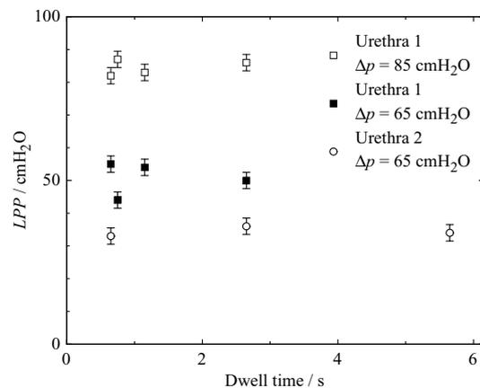
Fig. 4. *LPP* to close a sow urethra does not depend on the plateau times longer than 0.65 s. The error bars correspond to the standard deviation.
