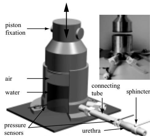
Fig. 1. Scheme of the bladder model system. The pressure impulse is lead through the connecting tube to the urethra. Two pressure sensors are fixed at the cylinder and at the end of the connecting tube, respectively.
