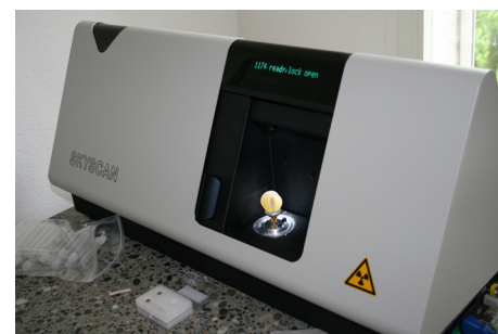
Skyscan 1174 (Skyscan Belgium) with 50 kV acceleration voltage and 800 mA beam current.
