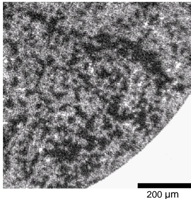
Fig. 3. Section of an absorption tomogram using synchrotron radiation (Pixel size: 2  $\mu\text{m}$ ).
