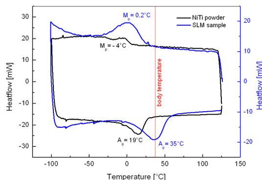
Fig. 4: DSC curves of NiTi powder and a SLM fabricated sample.
