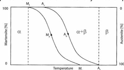
Fig. 1: Proportion of austenite  $\beta$  and martensite  $\alpha$  phases in dependence of the temperature.<sup>1</sup>
