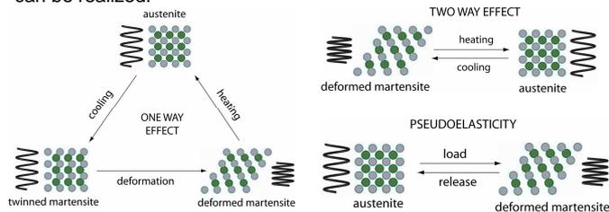
Fig. 2: Different effects in shape memory alloys.
