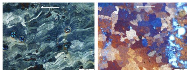
Fig. 6: Optical micrographs of the microstructure in SLM fabricated samples. Left: microstructure in the specimen, right: microstructure of supporting material. Arrows indicate building direction.
