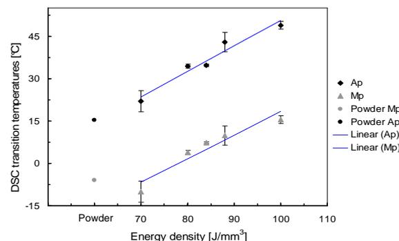
Fig. 5: Austenite and martensite peak temperatures of SLM samples fabricated with different energy densities of the laser.
