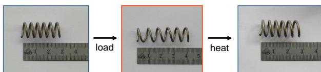
Fig. 3: One-way shape memory effect in SLM fabricated spring.
