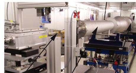
specimen flight tube detector
