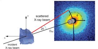
During the SAXS measurements at the cSAXS beamline the X-ray beam was focused to a spot size of 5 x 20  $\mu m^2$ , whereas the PILATUS detector was placed at 7.2 m distance from the specimen (D<sub>sd</sub>). For histological slices mounted on conventional microscopy glass plates an energy of 18.58 keV and for the slice
