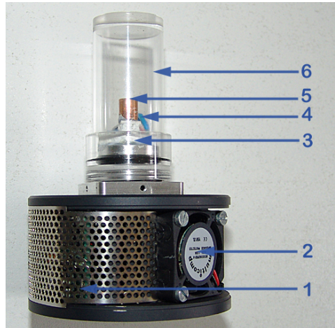
Figure 3. Photograph of heating stage consisting of (1) microprocessor controller and power converter for the Peltier elements inside protective metal, (2) fans for air cooling, (3) square-shaped Peltier elements, (4) copper-made specimen support with temperature sensor element, (5) specimen holder, and (6) transparent polymer cap with sealing ring. 11
