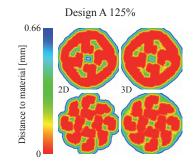
The pore size distribution can be determined by distance mapping. The 2D analysis slightly overestimates the distance to material compared to full 3D analysis. The distance histogram shows the compactness of the material. Clear differences between 2D and 3D analysis can be seen especially in the range above 2 mm.
