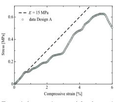
The steps in the stress-strain curve result from the successive cracking of the scaffold layers.
