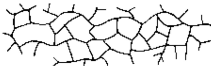
Figure 3: Example of constitution: Interconnected elastomers or duromers.
