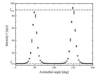
The degree of anisotropy is defined as  $(I_{\text{max}} - I_{\text{min}}) / (I_{\text{max}} + I_{\text{min}})$  which can be derived from the azimuthal intensity distribution. A strong orientation of the semi-crystalline lamellae stacks within the  $\mu$ C is observed for PVDF, POM and PP  $\mu$ Cs.
