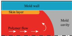
Filling of cavities is explained by fountain flow: solidification of melts at mold walls leading to skin layers.
