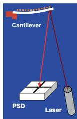
Cantilever sensing involves detection of cantilever bending. Adsorption of analytes onto the functionalised cantilever surface produces a differential stress between the two surfaces and induces bending.
