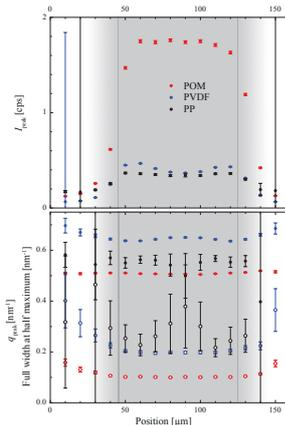
Variation of  $I_{\text{peak}}$ ,  $q_{\text{peak}}$ , and  $\text{FWHM}_{\text{peak}}$  across the central part ( $\mu$ C width in gray). The low intensity variations in the central part of the  $\mu$ C indicate a homogeneous semi-crystalline structure.
