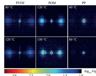
The distance of the spots from the beam stop is material dependent and decreases with the mold temperature [3].
