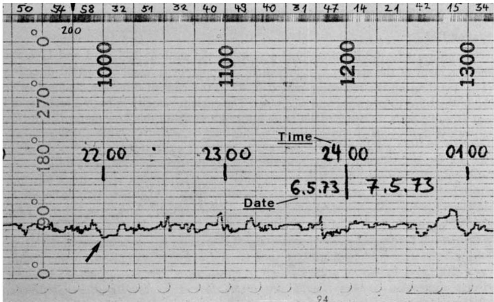
Fig. 11. Part of the original record obtained from station L-3 (Linth delta). Speed is determined by number of ticks per time interval (top of record). Note the periodic 'bunching' of ticks indicating pulsing flow character. Direction of flow is given by the position of the solid line (arrow) on the paper tape. Note the typical current caused oscillations.
