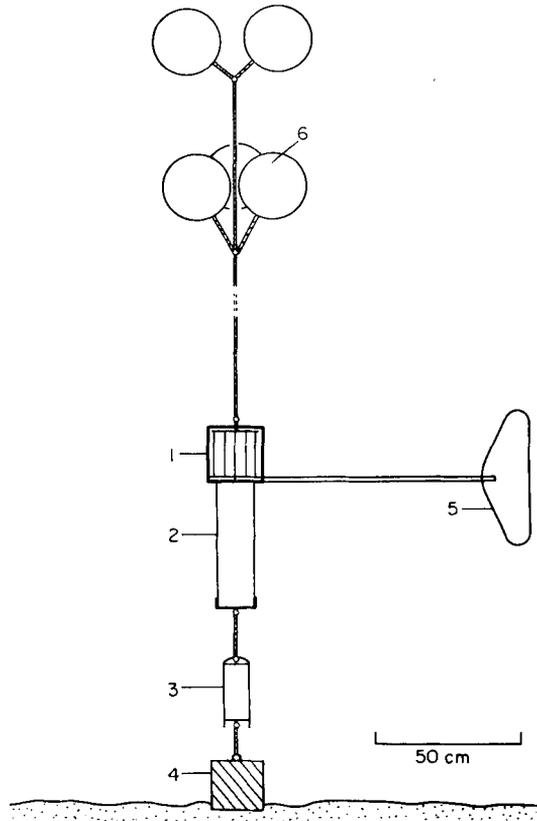
**Fig. 1.** Configuration of Scripps current meter (Isaacs-Schick-type) on the lake floor. 1, Housing with Savonius rotor; 2, electronic recording and compass packages; 3, automatic release; 4, concrete weight; 5, direction sensor van; 6, glass floats.
