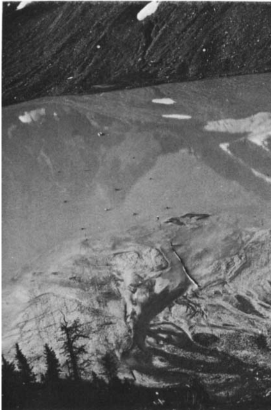
Fig. 5. An aerial view of the 3-D network in place. The individual stations were shifted about in order to adjust to changing input conditions. Small marker floats are also visible. They provided reference points for tracking the surface movement of the currents. The distal raft indicates the location of an electromagnetic current meter which was used to monitor movement beyond the grid.
