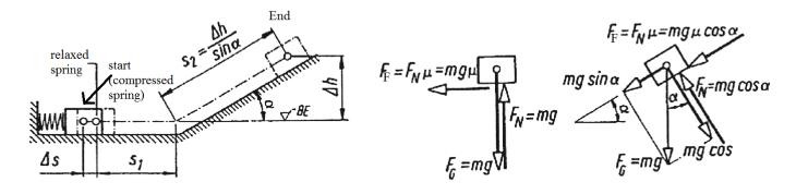
b) The energy at the end of the movement  $E_E$  is equal to the kinetic energy  $E_A$ , at the beginning, minus the loss due to the friction:
