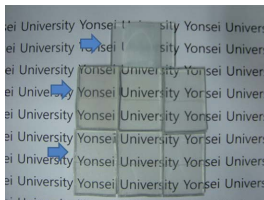
Fig. 4 Pictures of TiO 2 photoelectrodes; (top) commercial TiO 2 , (middle) mesoporous TiO 2 films at [TTIP]:[HCl]:[H 2 O] = 2 : 1 : 0, and (bottom) mesoporous TiO 2 films at [TTIP]:[HCl]:[H 2 O] = 2 : 1 : 1.
