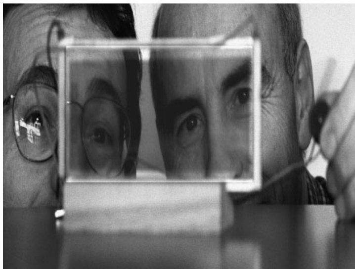
Figure 12. see-through DSC producing electric power from diffuse light to drive a fan
