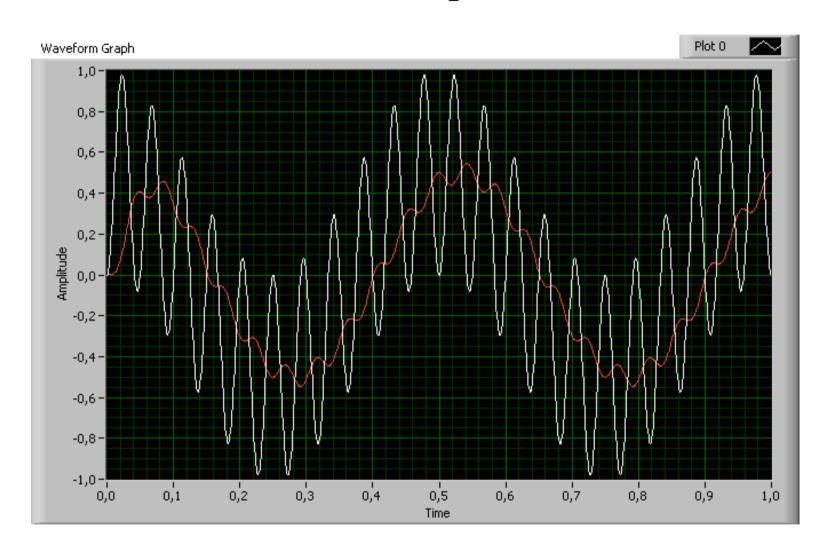
$f_1$ =10Hz  $f_2$ =12Hz  $\Phi$ =90°  $f_L$ =7Hz
