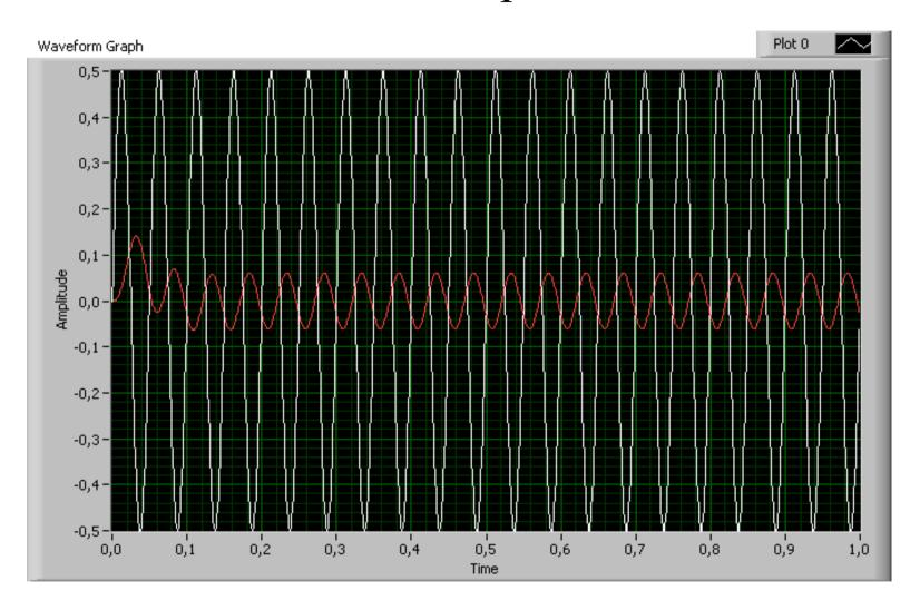
$f_1=f_2=10$ Hz  $\Phi=90^{\circ}$   $f_L=7$ Hz Butterworth 2
