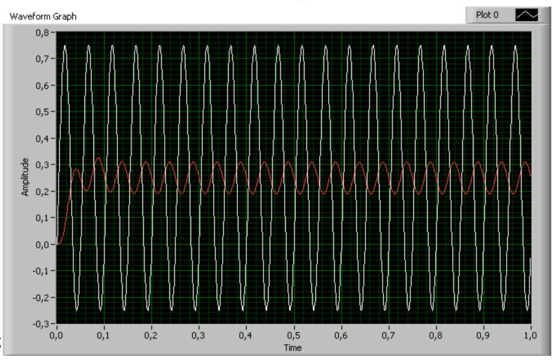
$f_1 = f_2 = 10$ Hz  $\Phi = 60^{\circ}$
